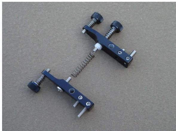
We are now ready for the final assembly. Locate the 1/8" dowel pins & #5 washers. Slide a dowel pin in each of the 1/8' reamed holes in the center of the base near each outer edge. Make sure there is no debris in the holes, they are a very close fit to the pins, less than 1/2 of one thousandth of an inch clearance. Slide one of the #5 washers over each pin.
