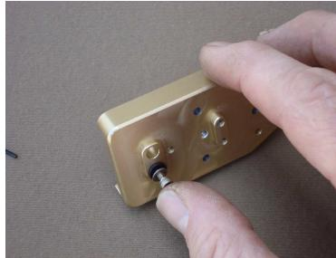
Turn the base over & slide a solder lug & #4 nut over the SHCS & snug the nut down.
