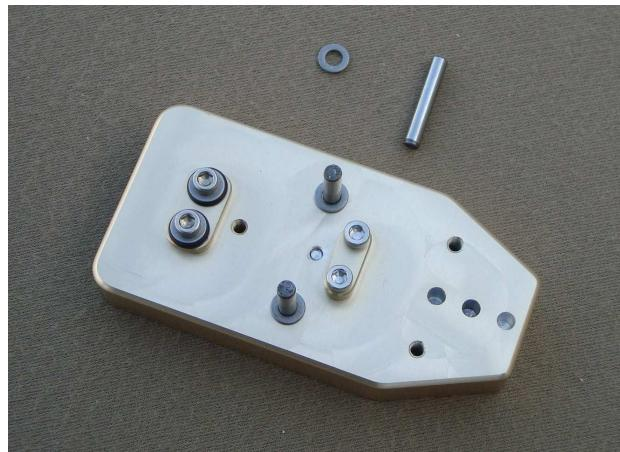
Now slide each of the levers onto it's corresponding pin, noting the orientation.
