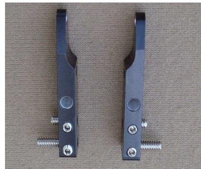
Now locate the remaining parts of the right lever. Note that it uses two of the 4 springs provided in the kit. To separate the springs, line them up together. There will be one long spring, two similar shorter springs, and one slightly longer than the two similar shorter springs. The two similar springs each fit on the two contact thumbscrews; the slightly longer one goes under the Return Adjust Thumbscrew head, and the longest spring is the return.
