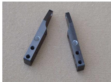
The Levers are pictured in their orientation when installed in the paddle; the "Right" lever has the step milled in the "left" side of the lever and the opposite for the "Left" lever.
