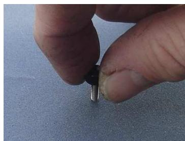
Locate the four shoulder washers, two #4 x 1/2 SHCS, two #4 nuts, and two #4 solder lugs. Push the washers into the corresponding holes in larger boss in the paddle base.
