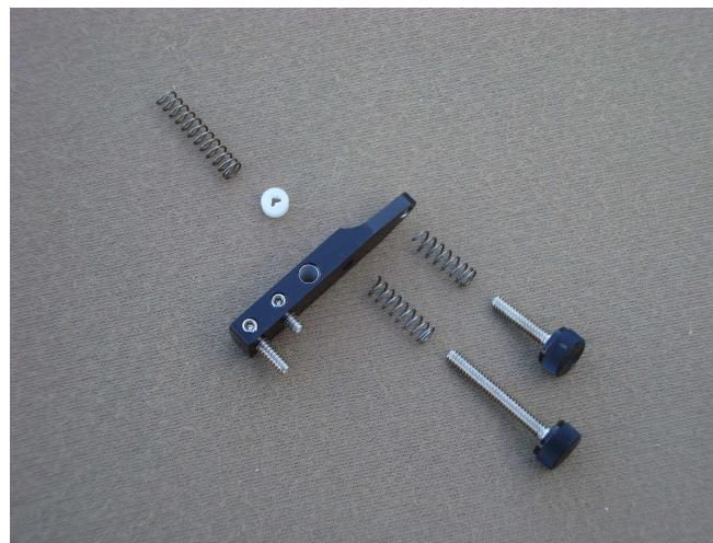
First please slide the middle size spring onto the Return Adjust Thumbscrew. Note that all springs have a closed end and an open trimmed end. The closed
