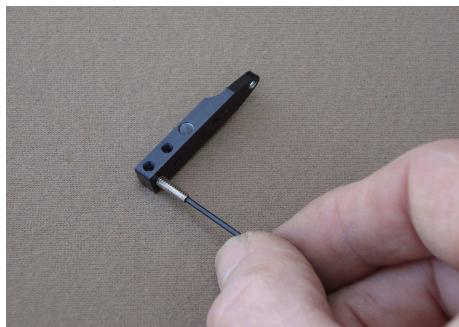
Note that the screws are threaded into the lever from the outboard or flat side of the lever.
