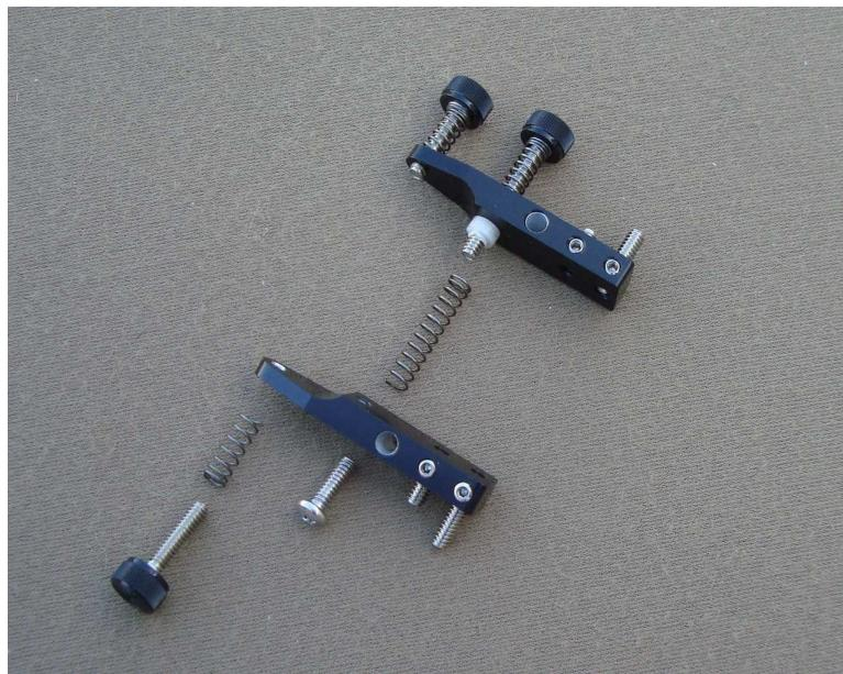
Do the same for the left lever Contact Thumbscrew, threading it into the left lever. Locate the #4 x 3/8 Pan Head Screw and thread it into the left lever center hole corresponding to the Return Adjust Thumbscrew on the right lever.
