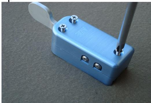
Use a #1 Philips screwdriver to adjust gap & spring. You can change the paddle lever ratio at any time by simply removing the top cover and moving the paddle dowel pin to the other hole. Nothing else will change when dowel pin is repositioned. Adjustment may be made at any time with a Philips screwdriver; the set screws with Delrin inserts will maintain adjustment.
