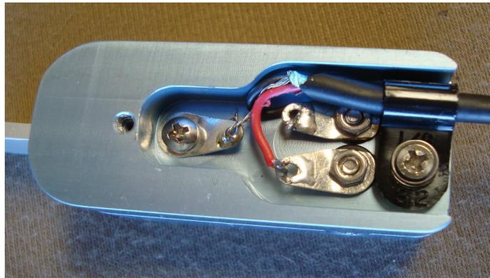
A 4-40 tapped hole is provided to mount the Mini-B; it will fit on the Desk Base, Qwikmount, and Leg Mount offered by American Morse Equipment. You can also bolt it to your rig or any other convenient mounting point with the #4 screw provided. For Sideswiper use, simply short together the left & right lugs.
