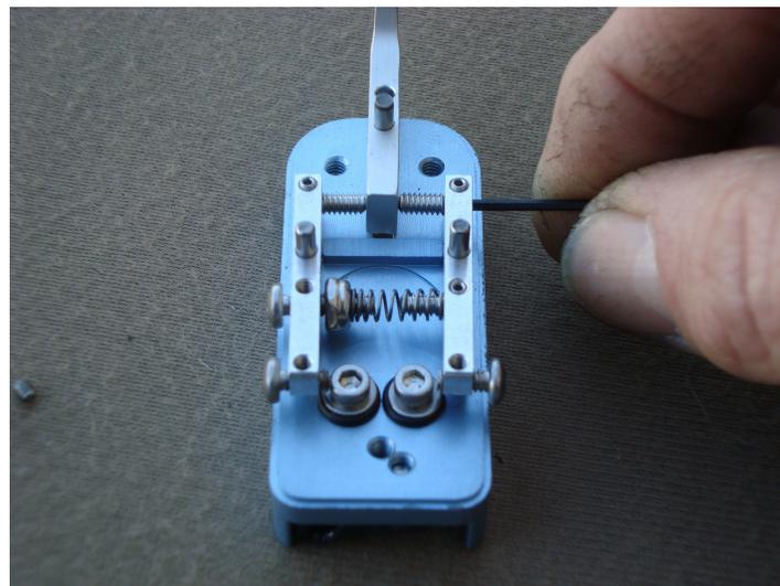
Using a #1 Philips screwdriver, turn in the contact screws until they almost touch the SHCS contacts - final adjustment may be made later, as well as spring force adjustment.
