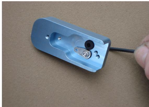
Repeat with the second cap screw. Now find the #4 x 3/16 pan head screw and the third, untrimmed solder lug, and secure the lug to the grounding hole in the underside of the base.
