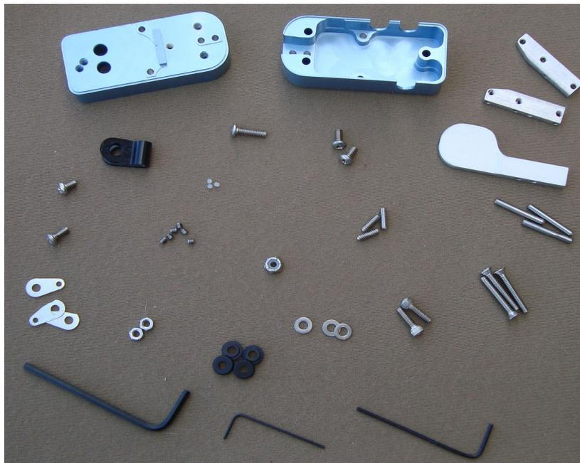
Once you have checked the parts inventory, you are ready to begin assembly. PLEASE NOTE: This kit is fully machined and all parts will fit together without excess force. If a pin doesn't fit a hole or whatever, do not force it - no hammer (Yikes!) needed! Check for metal chips, etc., if something does not go together. Please contact us with any problem. <[dwhauff@digitalputty.com](mailto:dwhauff@digitalputty.com)>
