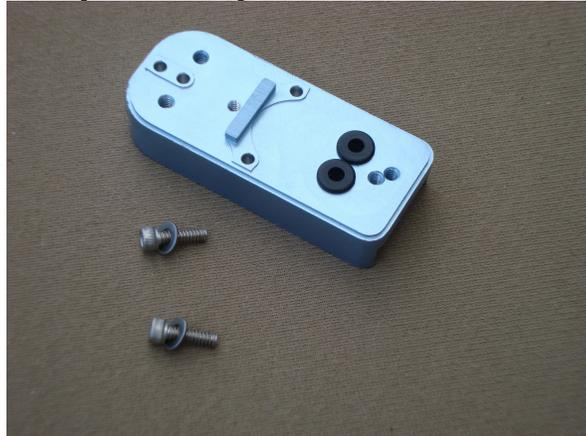
Put a flat washer over each of the two socket head cap screws. Insert one thru the top of one of the shoulder washers and thru the corresponding washer in the bottom; from the bottom slip one of the trimmed solder lugs over the screw, with the flat facing the adjacent hole, & secure with a #4 nut.
