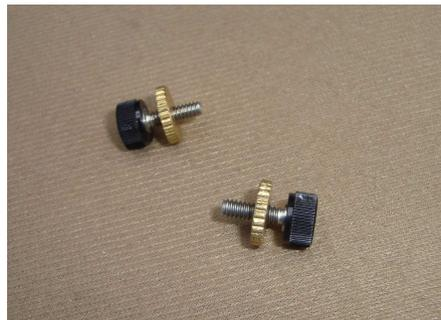
Screw the thumb nut assemblies into the remaining hole in the lever, and into the lever stop. Go ahead and set the spring compression and the contact gap with the thumb screws.
