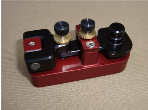
Turn the key over; you can fasten the cable stay to the base with the 1/4" pan head screw and #4 washer, or wait until you solder your 1/8" cable to the lugs.
