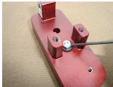
Tighten securely with the Philips screwdriver and a 3/16" nut driver or needle nose pliers. Note the position of the solder lug as you tighten the screw.
