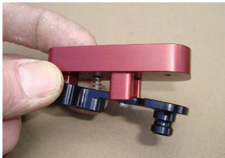
Turn the assembly over, and holding the assembly with one hand, insert the dowel pin into one side of the lever and thru the base, then thru the other side of the lever. It's not hard; just push the pin into the lever and against the side of the base, and while applying gentle force to the end of the pin, move the lever around to align the holes. The pin will find its way into the hole and line things up.
