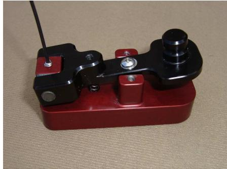
Using the two #4 flat head screws, fasten the lever stop to base.
