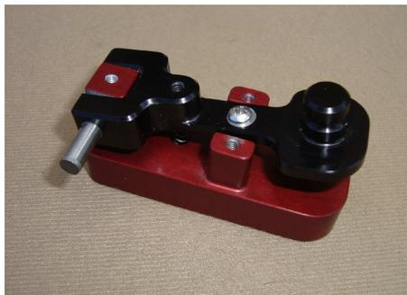
Find the #4 set screw and the .050" Allen key. Center the dowel pin in the lever, and clamp the pin with the set screw.
