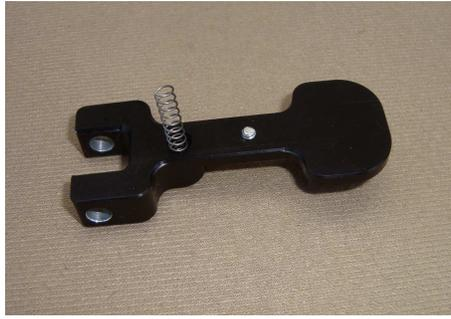
Holding the lever in the inverted position, present it to the base, guiding the spring into the corresponding hole in the base as you slide the lever clevis over the pivot boss on the base. Slide the lever over the boss until the 3/16 diameter cross holes are reasonably lined up.
