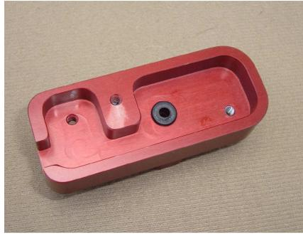
The top of the hole is harder to access due to the lever stop support bosses; too narrow for your fingers. Use the side of the screwdriver shaft or other suitable blunt object to push the washer into the hole; again you will feel (and easily see) when the washer seats.
