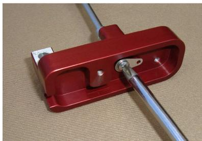
Find the 3/16 pan head screw with the unground end and put the remaining solder lug over it, and screw it into the base near the corner of the pocket, again noting the
