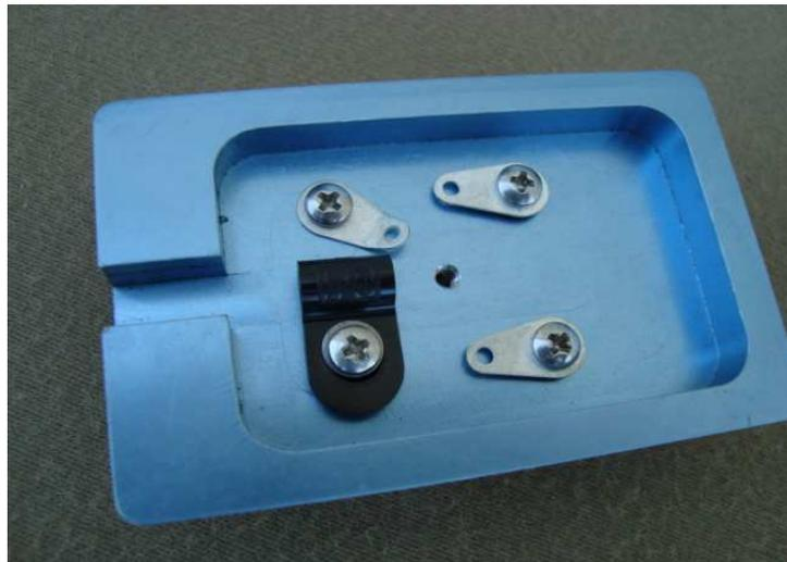
Next is to prepare the levers. Screw the shorter ground end ¼ pan head screws into the holes nearer the paddle finger surface. Thread the thumb nuts onto the four thumbscrews, and screw them into the remaining two holes. Thread two standard nuts onto each of the end thumbscrews. With the bottom nut flush to the bottom of the thumbscrew, tighten the other nut to lock them to each thumbscrew.
