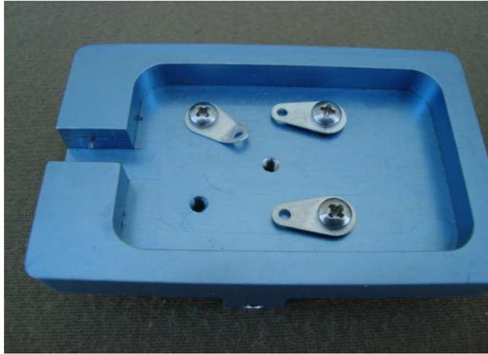
The other plain #4 x ¼ pan head screw and flat washer secure the strain relief. The base is now ready to receive the levers.
