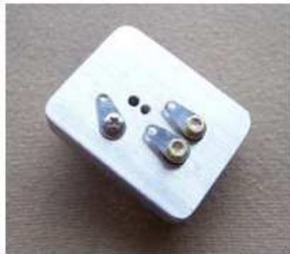
Turn the base back over & insert the two dowel pins in their holes & place one of the #5 washers over each, smooth side up.
