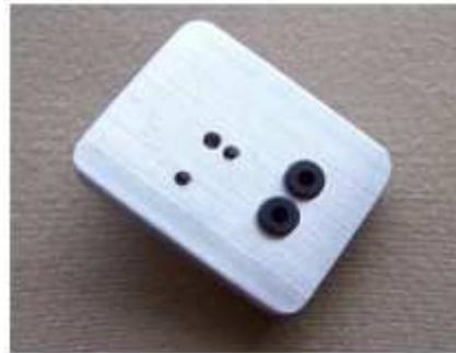
Now locate the two socket head cap screws, and after placing a #4 washer under the head of each screw, insert them through the top shoulder washers. Turn the base over and put a solder lug and 4-40 nut on each & tighten. Secure the ground solder lug with the 4-40 x 3/16 screw.
