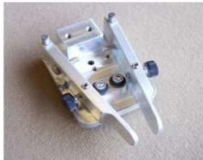
Locate the pin retainer & place it over the pins, locking in place with the two remaining 4-40 x 7/16 screws.
