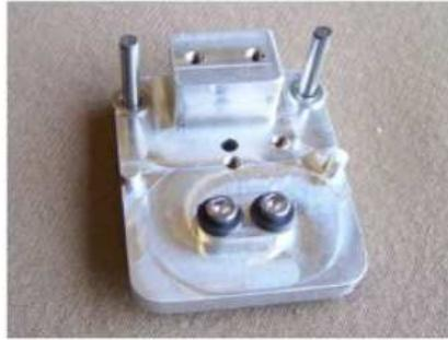
The base is now ready to receive the levers, so we'll prepare them next. Each lever gets one of the 4-40 X 7/16 screws thru the hole closest to the dowel pin bore. The other hole on each gets a thumb screw. Locate the 4-40 set screws and the .050 Allen wrench. Screw the set screw into the tapped hole at 90 degrees to each thumb screw.
