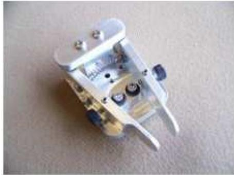
Turn the base over and install the plastic bumpers in the corners of the bottom of the base. Assembly is now complete; adjust the contact gap with the set screws, and preload the spring with the washers to your taste. Mount to rig or heavy base using either the 4-40 tapped or thru hole in the paddle base.
