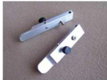
Slide each lever over it's respective dowel pin. Note the lever must fit inside of the lever stops integral to the base.
